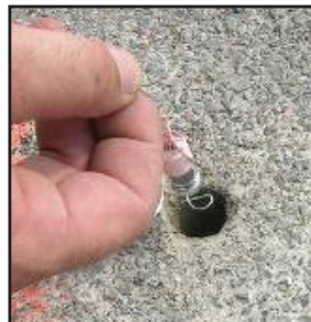
Sampler being deployed for sub-slab gas sampling
