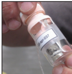
Sampler in a glass overpack for shipping
