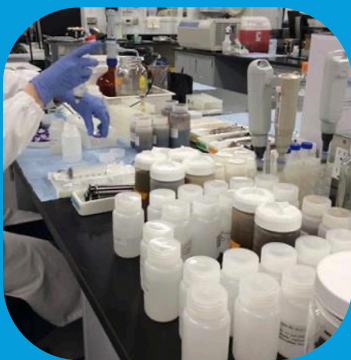
FIGURE 2: Different soil water ratios were tested to determine the partitioning coefficient ( K_d ).
